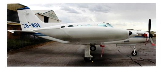
A Hendrik Venter & Company creation, customizing stock, Cessna 402, airplanes. Six, Cessna 'Falcon' 402 airplanes, have been modified since 2017 by replacing the twin piston engines on the wings with a single engine Walter M601D turboprop in the nose. The nose, then lengthened, to correct the center of gravity, increasing the payload, top speed & use on shorter runways. Two extra fuel tanks are added to the wings, giving the aircraft a much better flight range, over 800 nautical miles.
